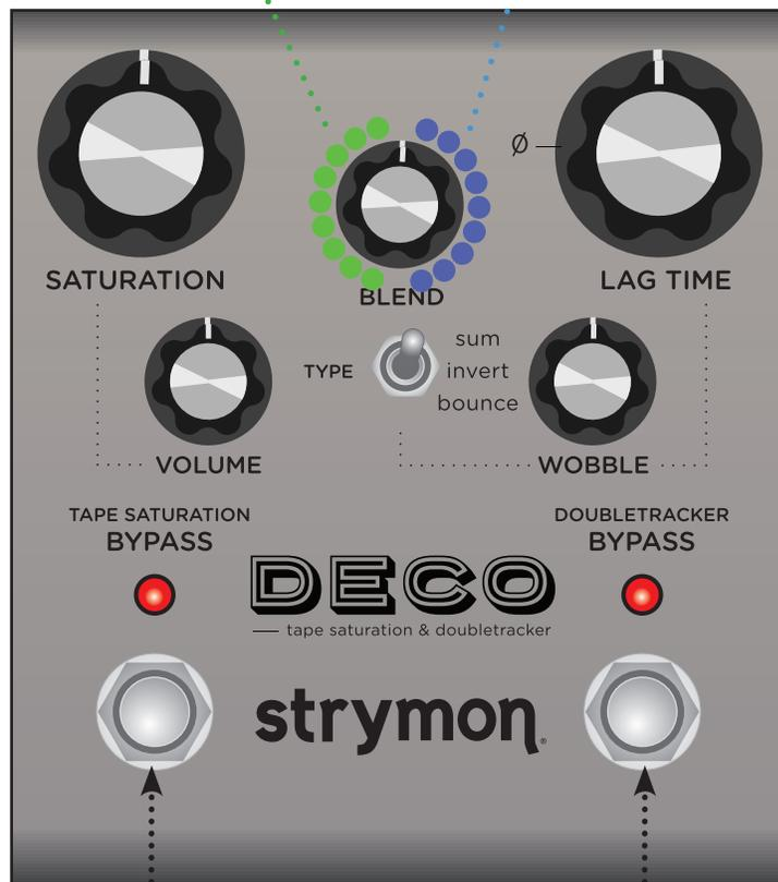
**HOLD BOTH AT POWER UP** while turning the BLEND knob to set Bypass Mode
