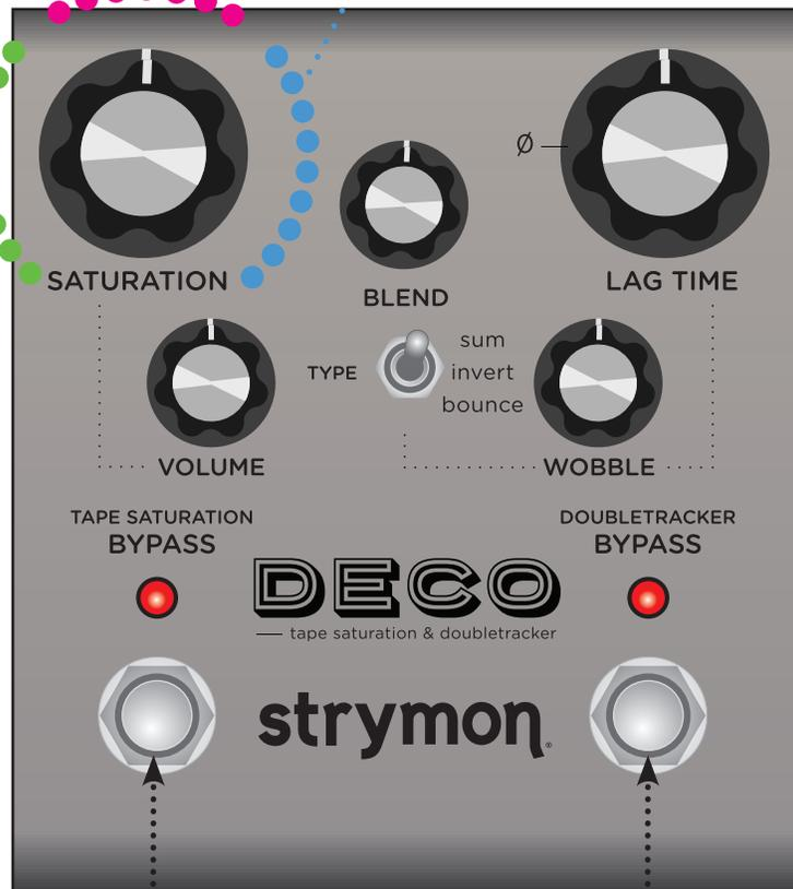
**HOLD BOTH AT POWER UP** while turning the SATURATION knob to set Expression Input Mode
