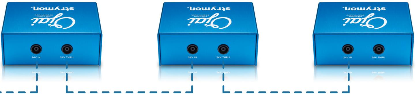
The included 24V power adapter provides a maximum of 24W, allowing you to link as many as 20 Ojai units together powered from one 24V power adapter. This configuration could theoretically power up to 100 low current draw pedals.
