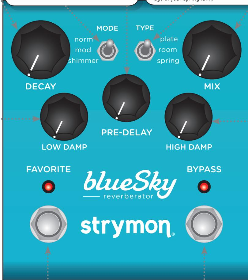
**FAVORITE FOOTSWITCH:** Press to select saved favorite sound. When **FAVORITE LED** is lit the favorite setting is engaged. When each knob is turned, the LED will indicate the saved favorite position of the knob. Push and hold the foot switch to save a new favorite sound.
