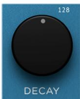
**DECAY** - Controls the decay time of the reverberated signal from very short to over 50 seconds. The size of the reverberated space is simultaneously expanded as the knob is turned clockwise.
