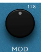
**MOD** - Adds a wide range of modulation to the reverberated signal. Modulation is off at the minimum setting.
