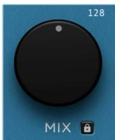
**MIX** and **MIX LOCK** - The **MIX** knob controls the mix from full dry at minimum to full wet (reverb + ensemble) at maximum. A 50/50 mix occurs at approximately 3 o'clock on the knob.
