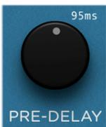
**PRE-DELAY** - Sets the amount of time before the reverberated signal appears, an essential control in creating an accurate and pleasing reverb. For most natural results, use lower **MIX** knob settings when using higher **PRE-DELAY**.
