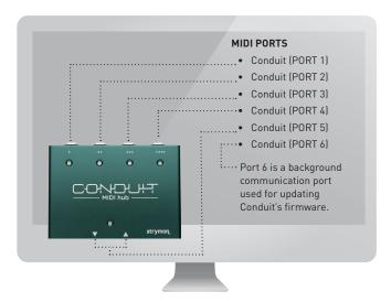
The diagram above shows how the MIDI ports corresponding to each of the devices connected to Conduit will show up in your computer/DAW.
