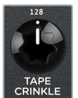
**TAPE CRINKLE** - Adjusts the amount and severity of tape irregularities, including friction, creases, splices, and contaminants. Tape Crinkle characteristics track accordingly to tape speed. Set to minimum for a fresh, clean tape. Set to maximum for a tape that has been
