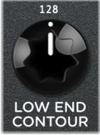
**LOW END CONTOUR** - Controls the low frequency shaping of the echo repeats. Set to minimum for extended low frequency bandwidth. Set to maximum for extremely high-passed, magnetic drum style repeats.
