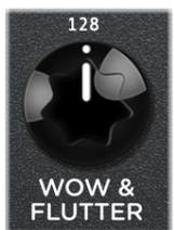
**WOW & FLUTTER** - Controls the amount of mechanically related tape speed fluctuations. This also results in natural tape-style modulation. Turn the knob to minimum for a perfectly tuned, cleaned, and serviced tape machine.
