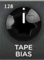
**TAPE BIAS** - Adjusts the bias of the tape machine, from under to over-biased. Higher bias levels result in reduced echo volume and limited headroom with dirty sounding repeats. Lower bias settings result in the cleanest echoes with the most headroom.
