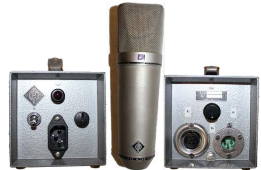
Neumann™ U67 in the U269 version with remote-controlled directional characteristic
