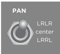
**PAN:** Selects between three different stereo panning modes for the tape heads. When only one output jack is connected, all head signals will appear at that output summed to mono.
