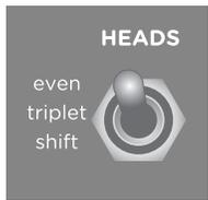
**HEADS:** Selects between three different modes for the tape heads. Even spacing, triplet spacing, and rhythmic shifted pitches.
