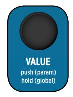
NAME: Allows editing the name of current preset. Use TYPE encoder to select a character. Use VALUE encoder to change the selected character. Exit by pressing the VALUE encoder. Hold the TYPE encoder to save the name.
