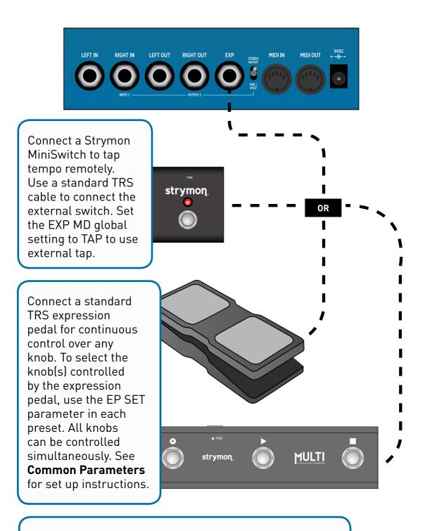
Connect a Strymon MultiSwitch for external tap tempo, bank selection, or preset selection. Set the EXP MD global setting to either TAP, BANK, or PRESET. Please refer to the MultiSwitch user manual for detailed setup information: www.strymon.net/support/multiswitch
