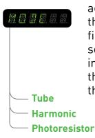
Selects the current tremolo type. The tube tremolo accomplished its tremolo sound by varying the bias on the output tube circuit. The harmonic trem used band filtering to achieve tremolo with a unique "phasey" sound. The photoresistor tremolo cut the amplifier in and out with a bulb/photoresistor combination for the most choppy and square sounding tremolo of the three.
