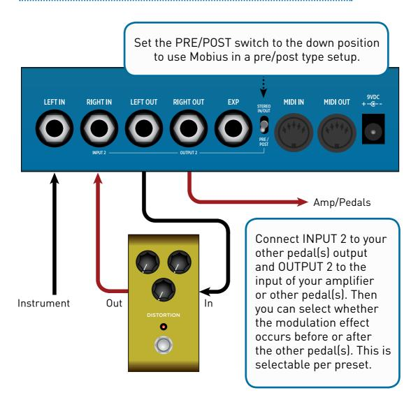
When connected as above, the PRE/POST setting in the preset menu has the following effect:
