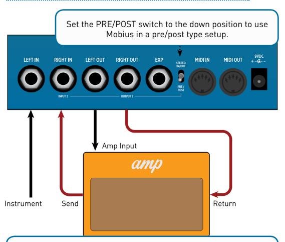
Connect INPUT 2 and OUTPUT 2 to your amplifier's effects loop. Then you can select whether the modulation effect occurs before the amplifier input or in the amplifier effects loop. This is selectable per preset.
