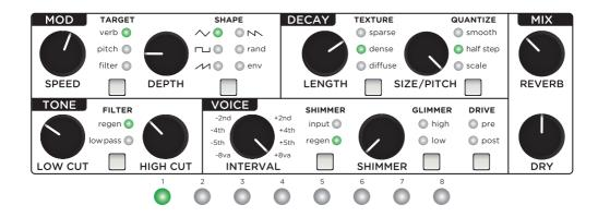
MIDI clock / MIDI exp: OFF Glimmer Gain: 12 o'clock Drive Gain: max Pre-Delay: 10'oclock Infinite Input: on Scale Select: minor pentatonic Low Pass Resonance: min Sequence Glide: min
