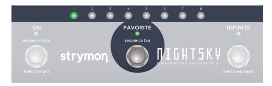
There are 16 onboard presets that are accessible by using the 8 **PRESET BUTTONS** on NightSky. They are arranged in 2 banks of 8 presets with different **PRESET BUTTON** colors indicating the selected bank.
