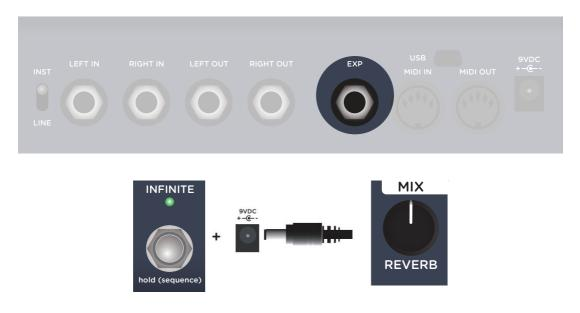
**Expression Pedal Mode: GREEN** - Allows continuous control over any of the knobs in any direction with a standard TRS expression pedal.
