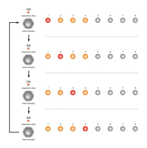
**NOTE:** If the sequencer is running, pressing the **ON** (sequence step) footswitch once will stop the sequence and return to the first step.
