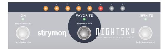
**NOTE:** A minimum of two active steps are required for the sequence to run.
