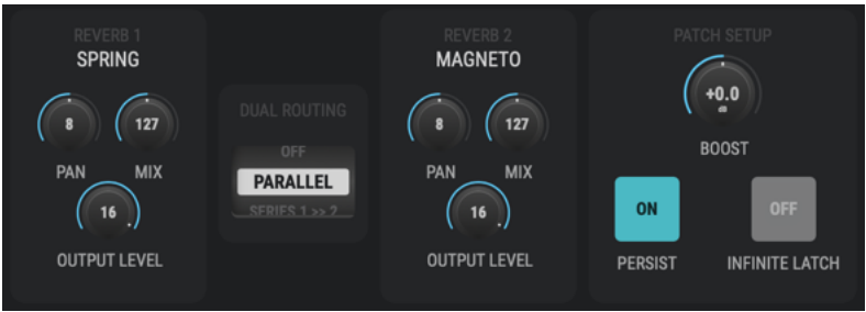
The Dual/Mixer parameter panel - Parallel Dual Routing selected
