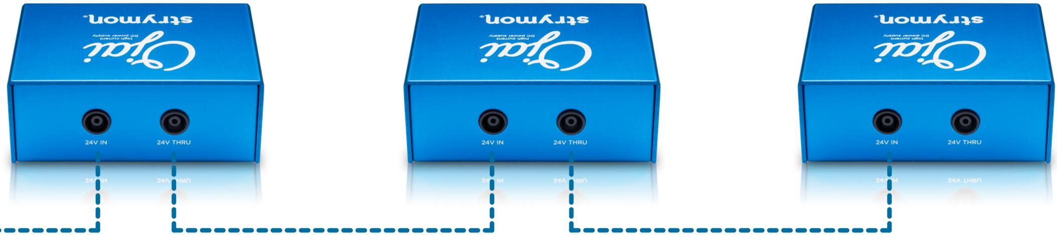
Ojai provides a huge amount of power. You can link together as many as 7 Ojai units powered from one 24V power adapter, powering up to 35 effects pedals. While it's unlikely that anyone would go to such extremes, we wanted to ensure Ojai delivers maximum flexibility and expandability. A much more likely scenario would be to link 2 or 3 Ojai units together, powering a combination of up to 15 high and low current draw pedals.
