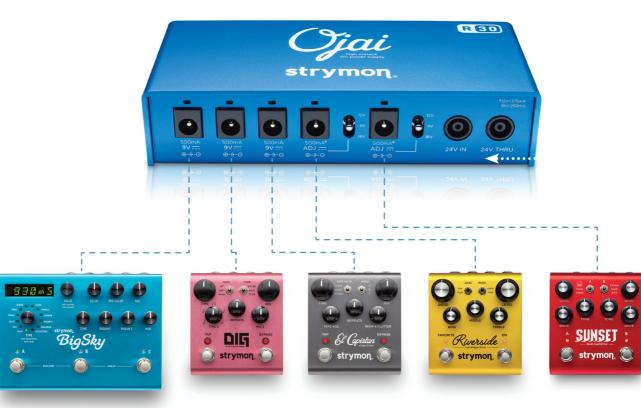
**NOTE:** Use non-adjustable outputs first to power your Strymon pedals. If using adjustable outputs with Strymon pedals, make sure these outputs are set to 9V.
