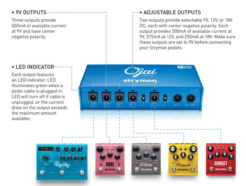
**NOTE:** Use non-adjustable outputs first to power your Strymon pedals. If using adjustable outputs with Strymon pedals, make sure these outputs are set to 9V.
