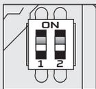
**Spillover:** Enables effect spillover between the Favorite presets and the manual setting of the module by setting rear dip switch 1 to **ON**.
