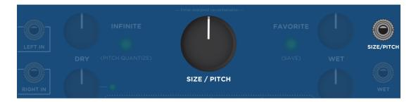
SIZE/PITCH CV: Modifies the SIZE/PITCH setting at 1V/octave. SIZE/ PITCH knob acts as an offset.
