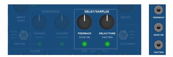
**FEEDBACK:** Applies regeneration to the delay, resulting in more repeats with longer delays, or more resonance with shorter delays.
