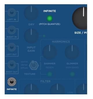
**INFINITE CV:** Engages the infinite effect to hold the input signal going into the reverb.
