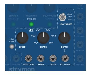
**LFO TARGET:** Selects one of three parameters that can be modified by the LFO.
