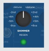
• To select the SHIMMER INTERVAL: Turn the SHIMMER knob while holding down the REGEN button.
