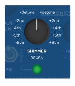
**SHIMMER INTERVAL:** Selects the interval of the pitch shifting shimmer effect. Turn the **SHIMMER** knob while holding down the **REGEN** button.
