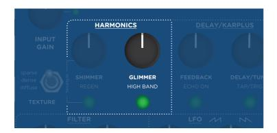
**GLIMMER:** Dynamically enhances aspects of the input signal's harmonic spectrum. Effect is OFF when **GLIMMER** knob is fully counterclockwise.
