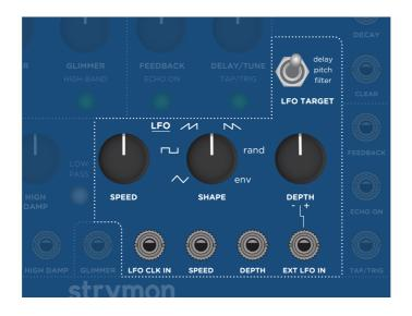
**SHAPE:** Selects from six different waveshapes for the LFO, including triangle, square, ramp, saw, random, and envelope which responds to input dynamics with the input sensitivity set by the **DEPTH** knob.
