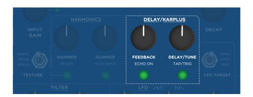
**DELAY/TUNE:** Sets string tuning over a continuous 4 octave range. When **SIZE/PITCH CV** is detected, it sets fine tuning of 12 semitones.
