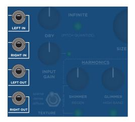
**LEFT/RIGHT IN:** Left and right audio inputs. Use **LEFT IN** for mono input.
