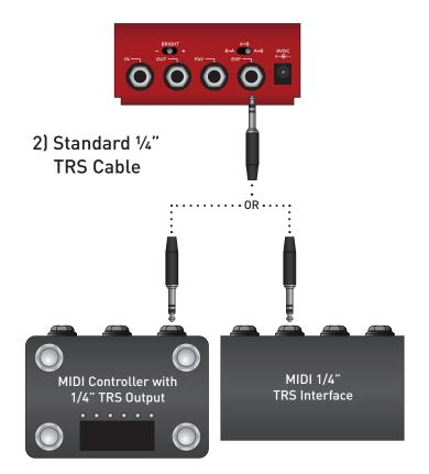
NOTE: If you are only sending data to Sunset - the most common configuration - the MIDI Output mode must be set to OFF. (See page 16 for details on configuring the MIDI Output Mode.)
