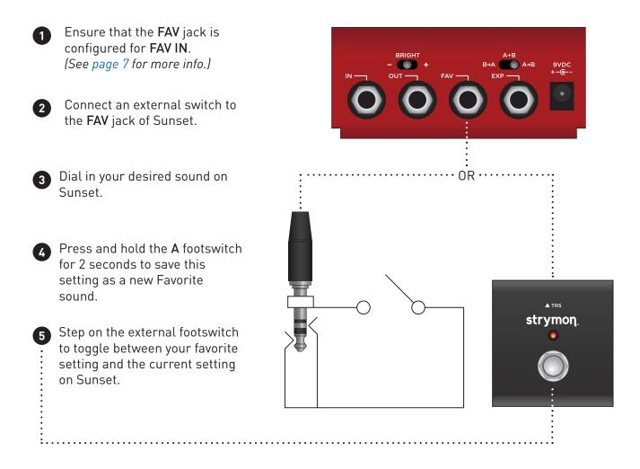
**NOTE:** Along with the knobs and toggle switches on the face of the pedal, the setting of the BRIGHT and CONFIG switches, the NOISE GATE and the bypass state of each side of Sunset is stored with the Favorite preset.
