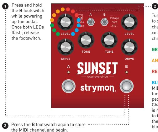
Turn the LEVEL knob on the A side to set the MIDI communication channel. The A LED will change color as the MIDI channel is changed.
