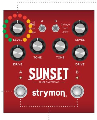
Turn the LEVEL knob on the A side to set the FAV jack mode. The A LED will change color to indicate the selection as the knob is turned.
