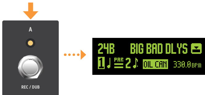
Overdubbing an existing loop (1 Button Looper)
