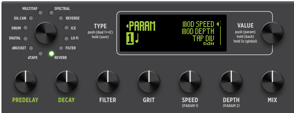
The Parameters menu and knob functions for the REVERB
