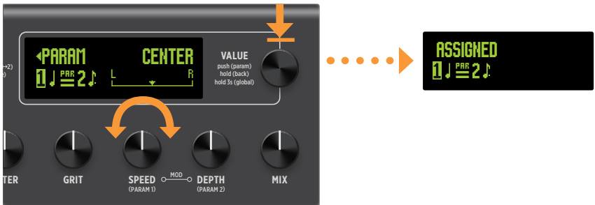
Assigning a parameter (Delay 1 - PAN) to the PARAM 1 knob
