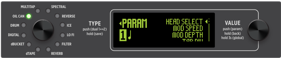
The Parameters menu (OIL CAN delay type is selected)
