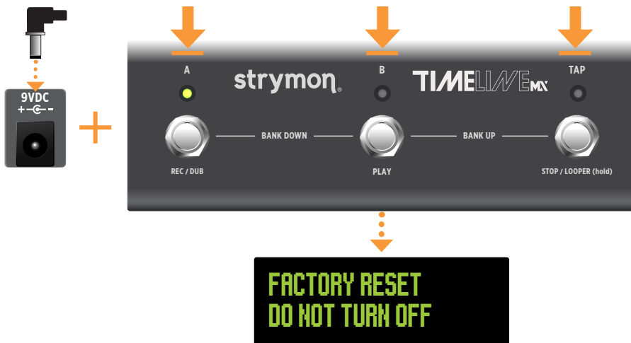
Performing a Factory Reset
