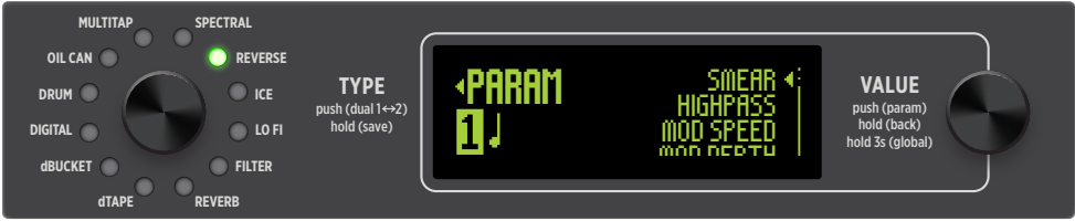
The Parameters menu (Reverse delay type is selected)
