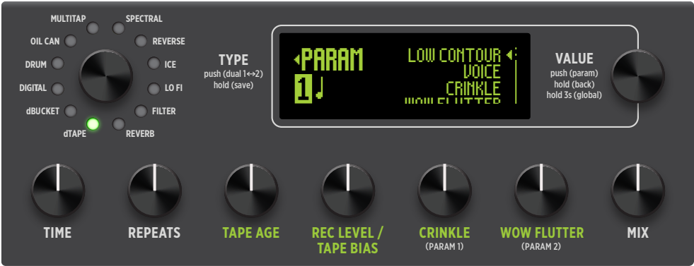
The Parameters menu and knob functions for the dTAPE delay type
