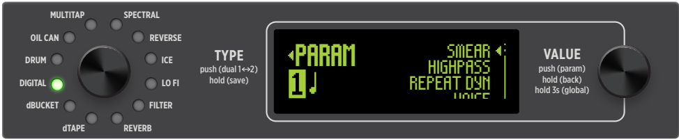
The Parameters menu (DIGITAL delay type is selected)
