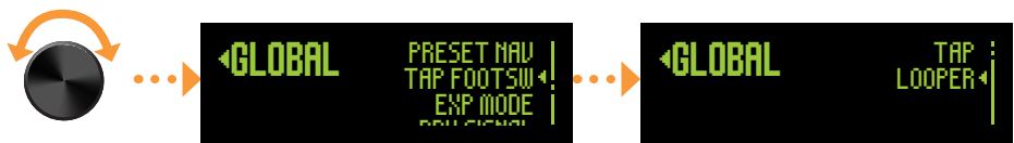
Configuring the TAP switch for 1 Button Looper functionality
