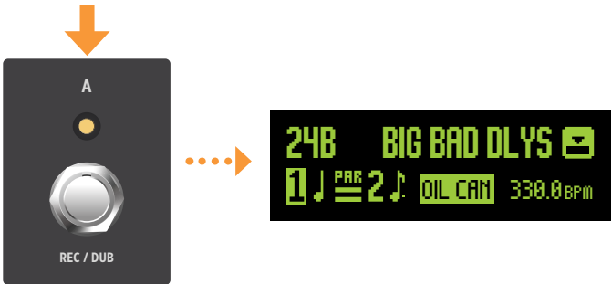
Overdubbing an existing loop (1 Button Looper)
