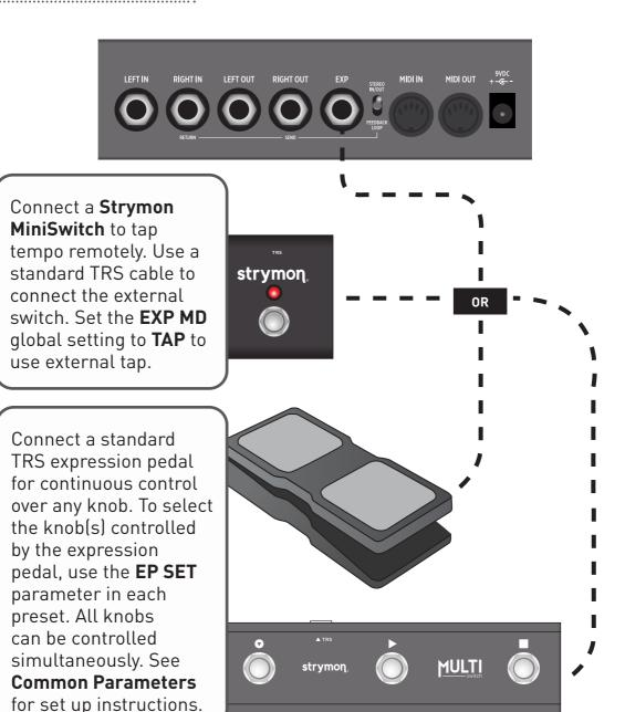
Connect a Strymon MultiSwitch for external bank selection, preset selection, or extended control of TimeLine's built-in looper. Set the **EXP MD** global setting to either TAP, BANK, PRESET, or LOOPER.
