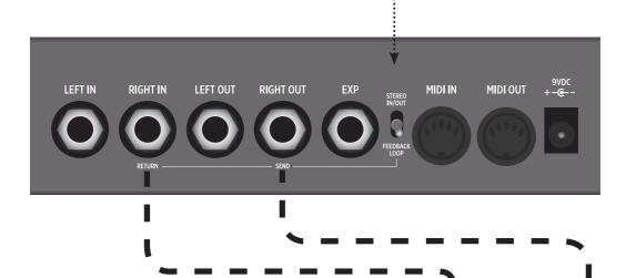
Connect an external effect to the feedback loop. Any external effect can be used. Feel free to experiment with the different sounds that can be achieved. All of the delay repeats will be processed through the external effect.
