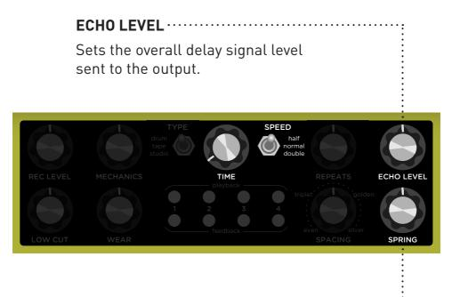
**NOTE:** The shortest possible delay time is achieved by setting **SPACING** to **triplet** and selecting head **1**.
