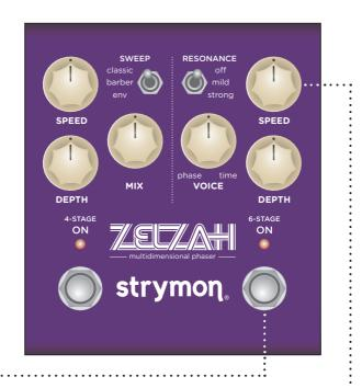
2 Turn the SPEED (6-STAGE) knob to select True Bypass or Buffered Bypass. The ON (6-STAGE) LED will change color to indicate the current status as the knob is turned.
