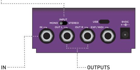
High impedance ultra lownoise discrete Class A JFET preamp input. Use a TRS stereo adapter/cable for stereo input. Low impedance stereo outputs. Use **OUT L** for mono output.
