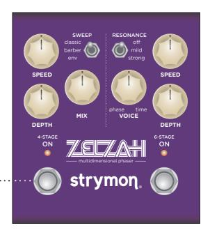
2 To save the current state of the pedal to the currently loaded preset location, press the **ON (4-STAGE)** footswitch.
