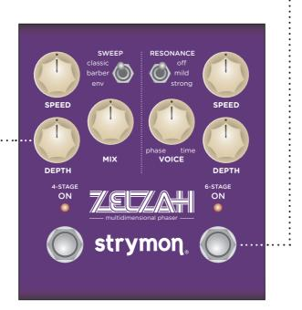
2 Turn the **DEPTH (4-STAGE)** knob to adjust the stereo spread of the 4-Stage phaser. Both LEDs will momentarily change color smoothly from **GREEN** (narrow) to **AMBER** (wide) to indicate the current status as the knob is turned.
