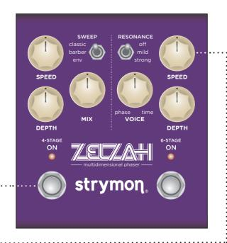
Turn the SPEED (6-STAGE) knob to select the function of the EXP/MIDI jack. ON (6-STAGE) LED will change color to indicate the current status as the knob is turned.
