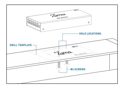
Drill holes. Drill through the two marked hole locations with a 1/8"
