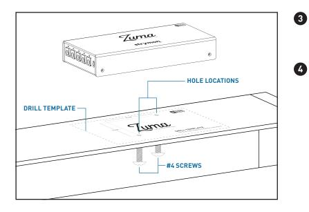
**Drill holes.** Drill through the two marked hole locations with a 1/8" (3mm) bit. Remove the drilling template.
