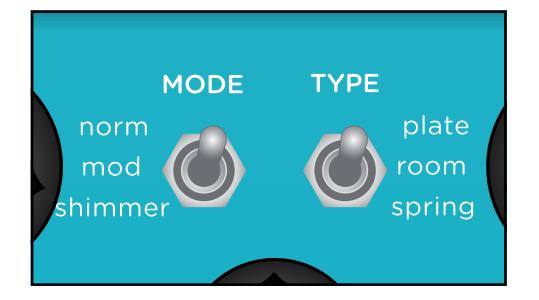
• MODE SWITCH Switches between 3 reverb modes (normal, mod, shimmer). Normal provides an unmodified version of the selected reverb type. Mod adds modulation to the selected reverb type. Shimmer adds regenerative octave up pitch shifting "in the tank" for a reverb trail that rises into the clouds with a Plate reverb. For Spring and Room shimmer, an octave plus a fifth is regeneratively introduced.
